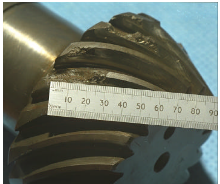
Figure 3 - Damaged input bevel gear teeth.
