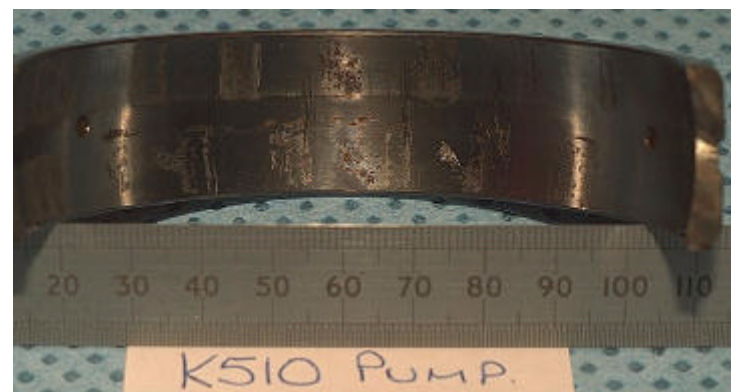
Figure 4 - Galvanic corrosion of the roller outer race.
