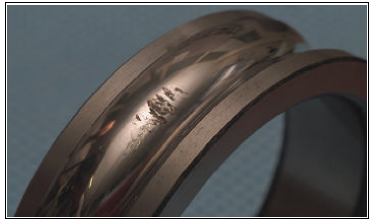
Figure 3 - Photographic evidence of bearing inner race defect.
