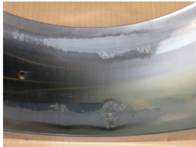
Figure 4 – Outer race defect found at drive side bearing.
