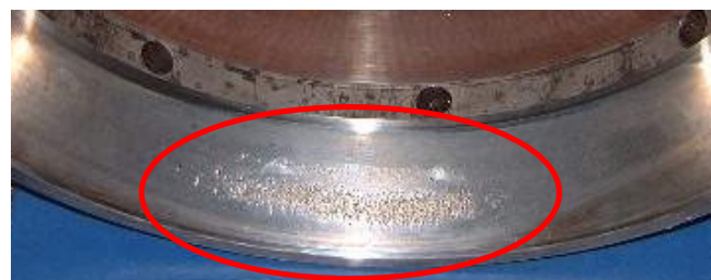
Figure 4 - Damage to roller bearing outer race.
