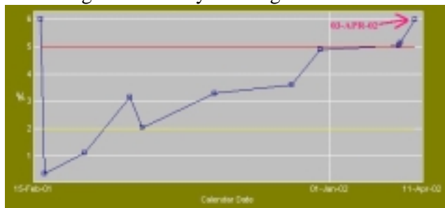
Figure 1 - Continued increase of overall vibration levels inboard bearing.
